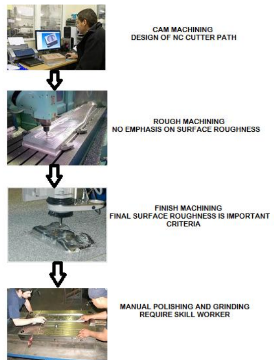
Figure 1.1: Current die manufacturing process sequence
